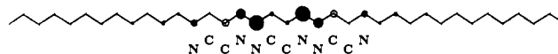
Figure 4. Calculated charge distribution of an isolated bipolaron in polyazine. The diameter of the circles is proportional to the amount of positive charge at that site. Closed circles are nitrogen atoms, and open circles are carbon atoms. Results are from the extended Hückel calculation of ref 40.
